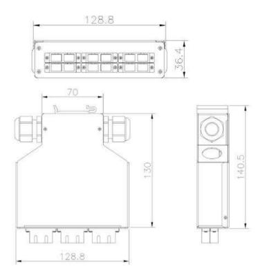
For 8 SC simplex adapters, 8 LC duplex adapters, 12 SC simplex adapters, 12 ST simplex adapters, 12 LC simplex adapters, 12 LC duplex adapter
