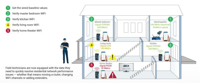
The figure above outlines the typical steps for installing a residential gigabit broadband service using the EX1.
